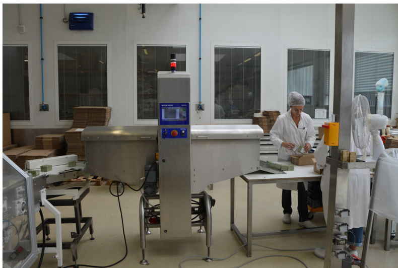
The X33 x-ray system inspecting Laboratoires BEA soap at the end of the production line before dispatch to markets worldwide.
